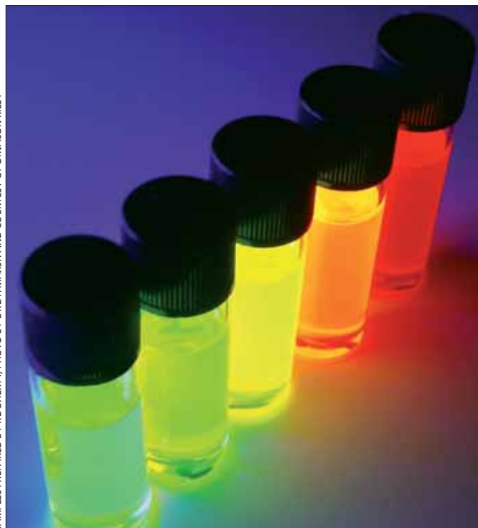
Fluorescence from capped CdSe nanoparticles in the 2–5 nm size range.
